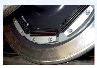
We offer different designs that allow radial and axial fixations on the wheels. Depending on the design the dampers will be mounted on the wheels or on carriers tensed in the wheel.
